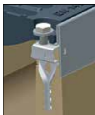
SECURE ANCHORING IN THE CONCRETE Fixing system designed by GRIDIRON: tang embedded into the concrete with a housing for the nut through which the screw is inserted
